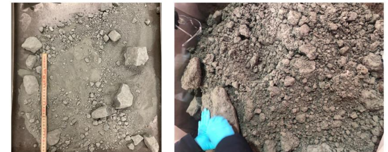
Figure 4. Sample of washed molasse (left) and wet molasse material (right) from Geneva Basin (Cern)
